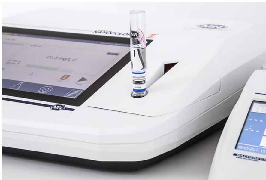
Quantitative determination of the generated CO<sub>2</sub> by an indicator (reaction basis analog to DIN EN 1484)
