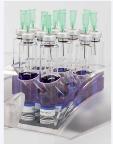
Oxidation of organic carbon compounds contained in the sample to CO<sub>2</sub>
